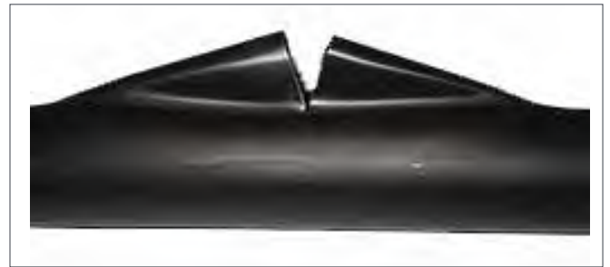
Figure 24: Pipe Failed in Ductile Mode
