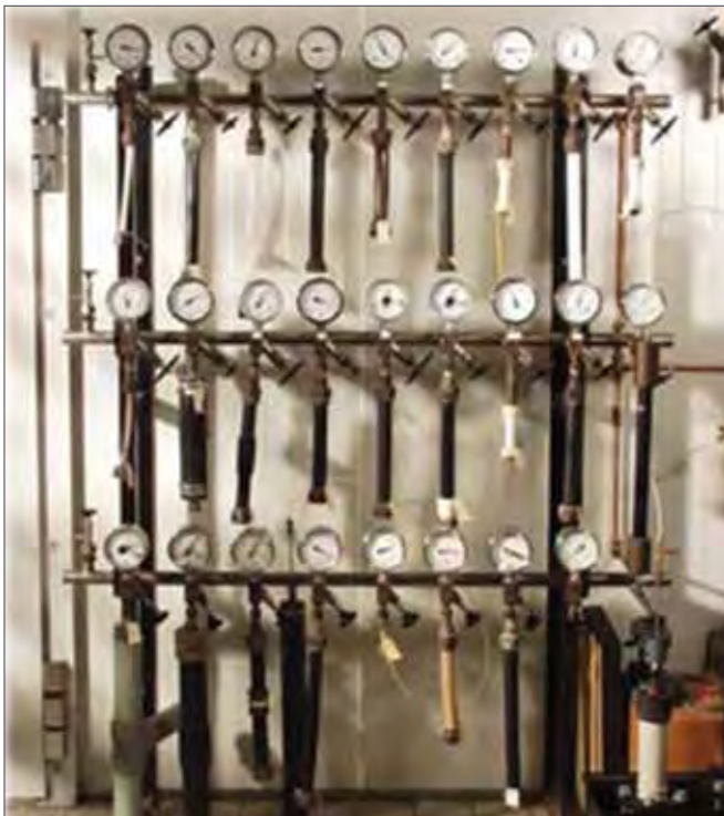
Figure 21: The First Creep Rupture Test Started in 1956 in HOECHST (today known as Lyondell Basell) Laboratory, Frankfurt, is still on test
