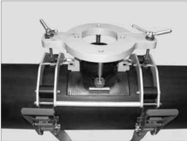
Figure 49: Illustration of Top-load Tool Attached to Both the Saddle and Pipe
